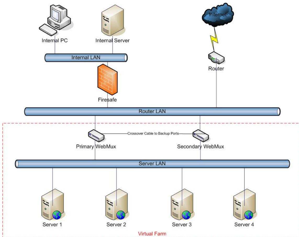
The main purpose of the WebMux™ is to balance the traffic among multiple web or other servers. The diagram above shows a NAT installation with two WebMuxes. In this configuration, one WebMux™ is serving as the primary, and the other is serving as the secondary, or backup, providing a fault tolerant solution.
