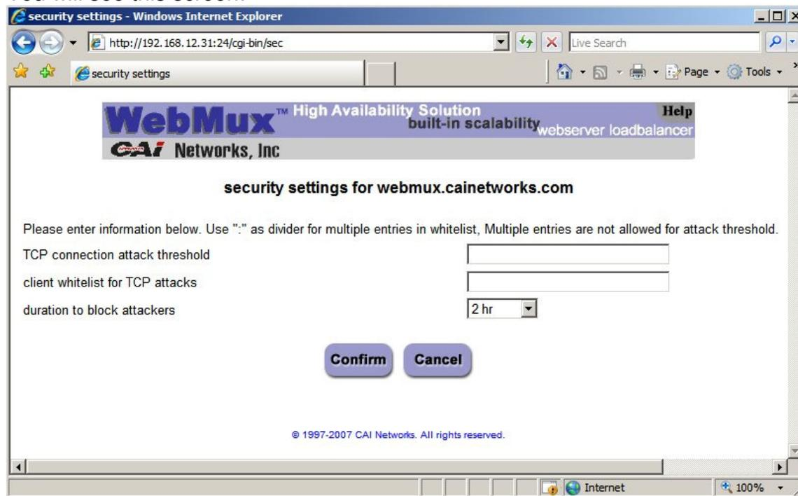
**TCP connection attack threshold:** This will set the maximum number of concurrent connection a client can make before the WebMux will consider it an attack. You do not want to set this value too low because most of time servers will experience several concurrent connections during normal operations. Usually a DoS or DDoS connection attack comes in by the hundreds. Set this value according to your needs.
