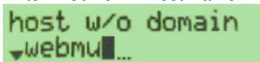
Enter the host name of the WebMux™. Use the right arrow to move the position, the up and down arrows to select characters, left arrow to move back in position, check mark button to confirm the change. This host name is for identification purposes. You may call it webmux1, webmux2, etc. (You can hold down the up/down button for more than a second to make quicker changes.) Note the left most down arrow on the LCD allows the user to move to other settings.
